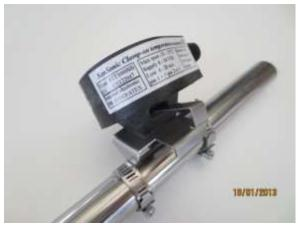
3. Press the spring down beneath the down bent edge and push it into.
