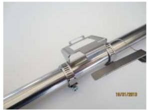
2. A) Apply heat conducting paste to the sensor. B) Hold the sensor obliquely towards the up bent edge. C) Insert the spring bar into the sensor mounting groove and further into the bracket's mounting groove.
