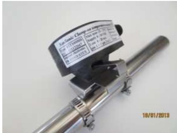
3. Press the spring down beneath the down bent edge and push it into.
